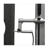
**Perpendicularity** Squareness measurements with electronic probe (V6)
