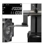
**Diameter Measurements** Simultaneous display of diameter and centerline
