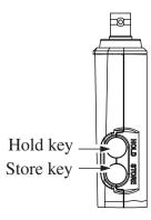
3. When the store key is pressed, the display very briefly turns off and the data are stored. The store address is incremented by 1 count. If the store address currently is 999 and the store key is pressed, the next store address will be 000.
