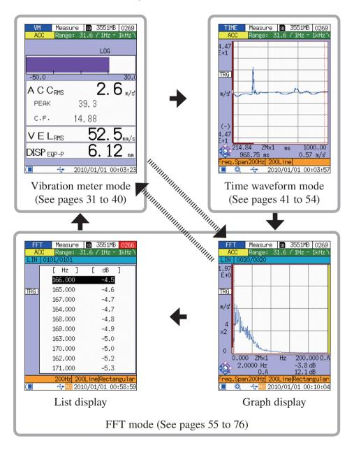
Because the time waveform mode and FFT mode (list display) are not shown in the default condition, the VM/TIME/FFT key operates as indicated by the broken arrows in the above illustration.
