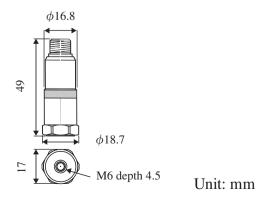
Supplied accessories: Piezoelectric Accelerometer PV-57I dimensional drawing
