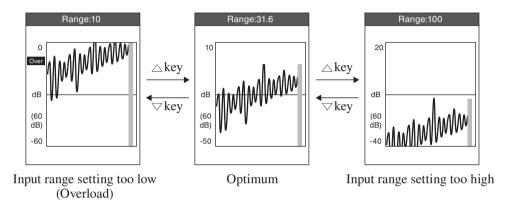
Relation between RANGE  $\triangle$  /  $\nabla$  keys and display (FFT scale is [Log])
