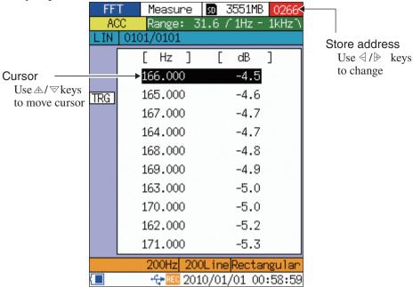
Pressing the VM/TIME/FFT key in graph display mode switches to list display. The ten highest level values out of the data range covered by the graph display are listed, in descending order.
