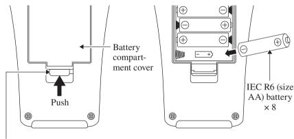
Push the latch in the arrow direction and then lift up to open the cover.
