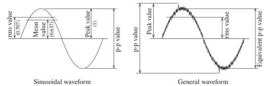
In case of a sinusoidal waveform, the peak value is the rms value  $\times \sqrt{2}$ . However, this does not apply for a general waveform.
