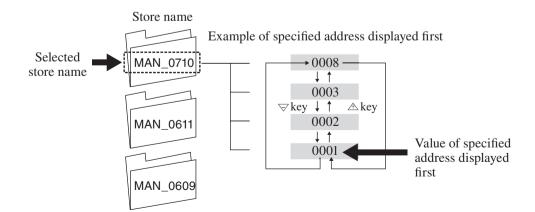
5. The data in the folder with the store name specified in step 3 and the store address specified in step 4 are displayed.
