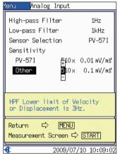
Use the  $\triangleleft/\triangleright$  keys to move to the item to change, and use the  $\triangle$  /  $\triangledown$  keys to change the numeric value.
