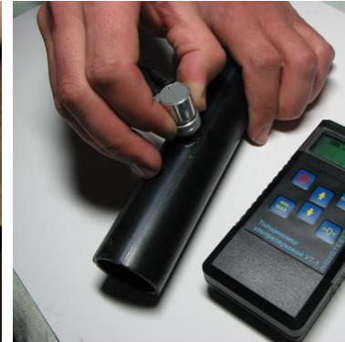
Measurement of wall thickness of the plastic pipe
