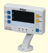
These displays show X and Y- axis coordinates with Retrofit Counter/DP Unit. (Can be switched between 1µm, 0.1µm, and 0.01µm)
