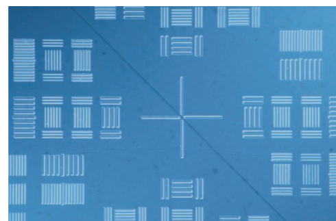
Left image: Semiconductor (IC wafer) (Objective: TU Plan Fluor BD 50x on Nikon Eclipse microscope)
