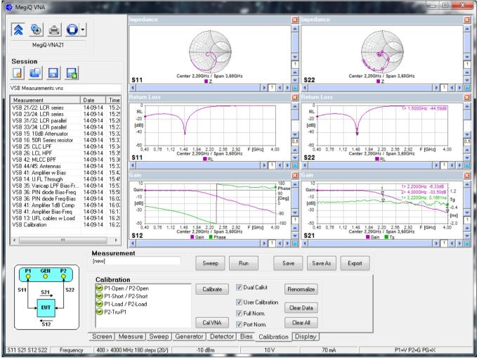
2 port measurement with impedance, return loss, gain, phase, group delay
