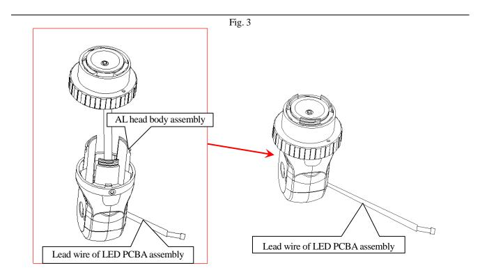
3 Pull out Lead wire of LED PCBA assembly through the hole of AL head body assembly as shown above.
