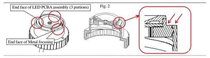
2 Align 3 portions of end faces of LED PCBA assembly and end face of Metal focusing ring.
