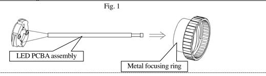
1 Pass LED PCBA assembly through Metal focusing ring.
