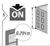
The result is shown in the main line and the measured distance above.
