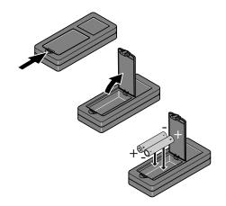
To ensure a reliable use, do not use zinc-carbon batteries.
