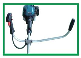
Designed so that the vertical center line of the handle bar stays aligned with that of user
