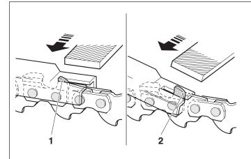
After having sharpened the chain, the height of the depth limiter must be checked by means of a chain gauge.
