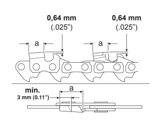
The sharpening angle ( $\alpha$ ) must be identical for all cutters!
