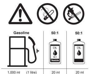
It is not wise to add more engine oil than specified to ensure safe operation. This will only result in a higher production of combus-tion residues which will pollute the environment and clog the exhaust channel in the cylinder as well as the muffler. In addition, fuel consumption will rise and performance will decrease.
