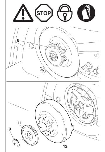
Check the sprocket before mounting a new chain.
