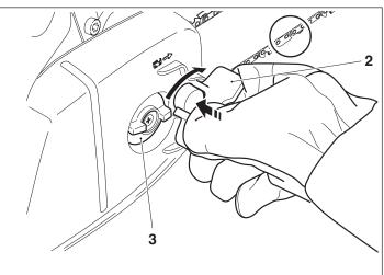
Release the sprocket guard chain tensioner until it turns freely, then fold it in between protective ribs (15) as shown in the illustration.
