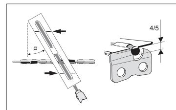
A file holder makes file guidance easier. It is marked for the correct sharpening angle of:
