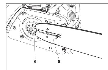
Put the guide bar (5) on and push it against the sprocket (6).
