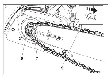
Lift the chain (8) over the sprocket (7).
