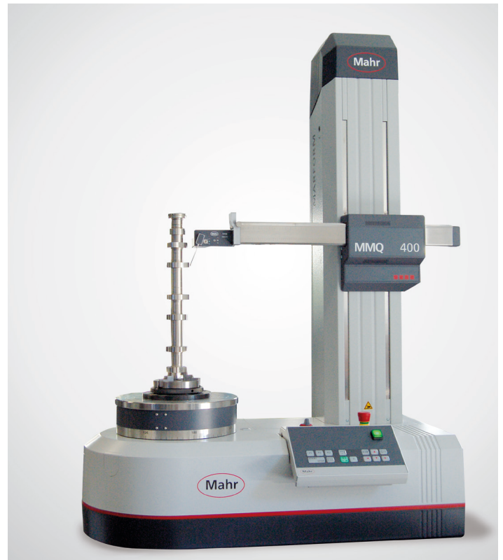
MMQ 400-2 with camshaft
