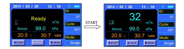
If under the Single Mode or B.P Mode, test will be finished and stop automatically. If under the Avg. Mode, it's necessary for finish testing by press "STOP" manually. When testing over under Single Mode or B.P Mode, press "SAVE" for testing data record. Or if under Avg. Mode for testing, data record of Auto save and Manual save can be optional.
