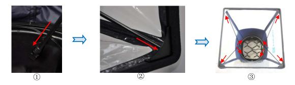
3) Micromanometer: installation procedure refer to the figures below: ①→⑤, and Figure ⑤ is the view of "After installation", unloading for remove is just reverse the steps.
