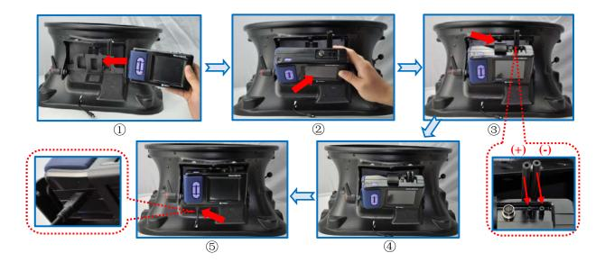
4) Portable handle: installation procedure refer to the figures ①②, After installation is just as
