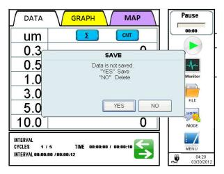
Tap [YES] to save the data. The calculation data will be created using the data collected before the power went out. Tap [NO] to discard the data.
