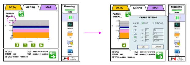
Select either LOG or LINEAR for the Y axis. Select the maximum scale value from four options. For setting the four maximum values, please refer to 3.8.1 MEASURING – CHART SETTING. In the display shown above, LOG is selected for the scale of the Y axis and the maximum scale value of the Y axis is set to 10 to the sixth.
