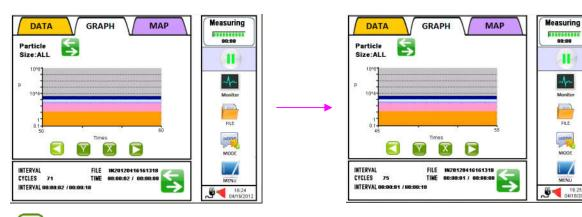
: Scrolls the chart to the right (half of the display can be scrolled at a time).
