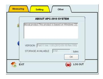
Tap [ABOUT] to view the firmware version of the instrument and the remaining capacity of the internal data storage.
