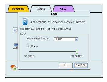
In the LCD settings, configure the Power saver time-out and Brightness setting. Also the LCD displays the power state of the unit (battery level, power source (AC/battery), battery charging, etc.).
