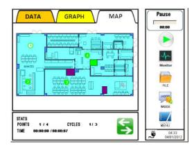
When a chart is displayed, users can change the particle chart to the ambient chart by tapping the button.
