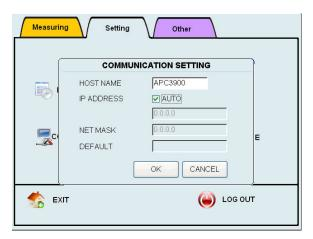
In the COMMUNICATION SETTING, configure the settings for Ethernet connection. This settings need to be configured when connecting the instrument to a PC using remote console or remote mode.
