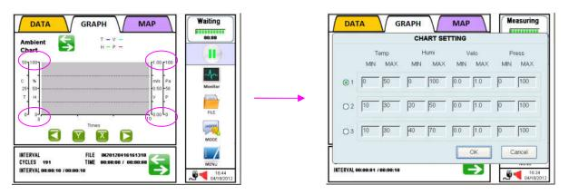
Select one of the three combinations of minimum and maximum scale values of the Y axis for each sensor. For setting the combination of minimum and maximum values, please refer to 3.8.1 MEASURING – CHART SETTING.
