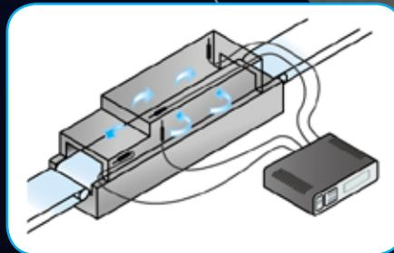
**Provide a real-time, complete picture of airflow characteristics in your production line or add an analog output module to the unit to facilitate automation**
