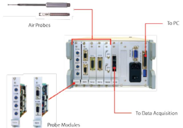
**A basic example of a complete multi-channel system**
