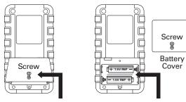
Lift up the battery cover with pulling the loosened screw.
