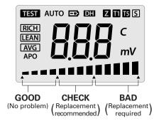
TEST : Lights up when the test is activated
