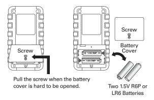
④Fix battery cover and tighten up the screw.
