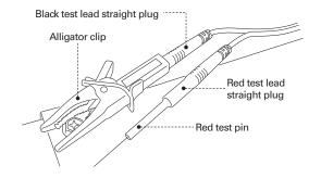
④Insert red test pin to the space of sensor signal cable from the backside of connecting couplers of O2 sensor or ECU (see "Confirmation of O2 Sensor Cables" and "Colors of O2 Sensor Cables" in page 17). Test procedures are the same as when using the check harness.
