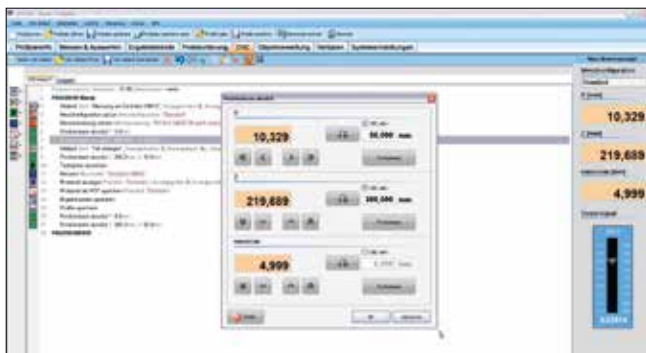
CNC editor for automated measuring runs
