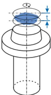
The tolerance zone is limited by two parallel planes at a distance  $t$  apart, which are perpendicular to the datum (rotational) axis. After several rotations around the datum axis and radial shift of the transducer, all points of the surface of the tolerance plane face must be within the tolerance zone.
