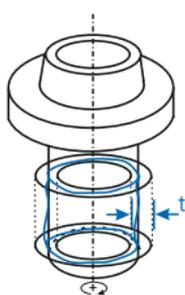
The tolerance zone is limited by two coaxial cylinders at a distance  $t$  apart, the axes of which match the datum axis. After several rotations around the datum axis and axial shift of the transducer all points of the tolerated element must be within the tolerance zone.
