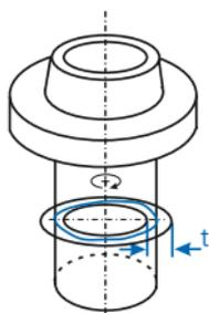
In every radial section plane perpendicular to the surface, the tolerance zone is limited by two concentric circles at a distance  $t$  apart, the common center point of which is on the datum axis. The radial run-out tolerance applies generally for a full revolution of the tolerated element around the datum axis.
