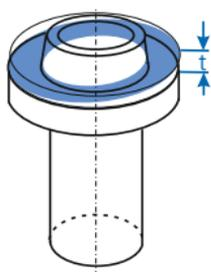
The tolerance zone is limited by two parallel planes at a distance  $t$  apart, which are perpendicular to the datum axis. The tolerated plane face must be between these two planes.
