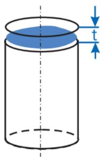
The tolerance zone is limited by two parallel planes at a distance  $t$  apart, the dimensions of which correspond to those of the tolerated area. The real workpiece area must be between the two parallel planes at distance  $t$  apart.
