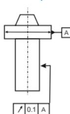
The circumference line of every radial section plane of the tolerated cylindrical area must be between two concentric circles at a distance apart of 0.1 with their common center point on the datum axis A.
