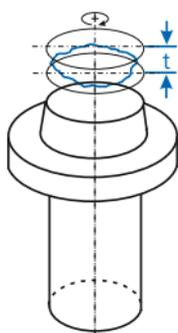
The tolerance zone is limited in every radial distance of two circles at a distance  $t$  apart. The circles are in a cylinder, the axis of which matches the datum axis. The diameter of the cylinder can adopt any value of the diameter of the plane face.
