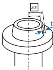
The tolerance zone is limited by two parallel planes at a distance  $t$  apart at the nominal angle to the datum axis.
