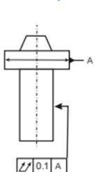
The tolerated cylindrical area must be between two coaxial cylinders with a radial distance apart of 0.1 with their common axis on the datum axis.
