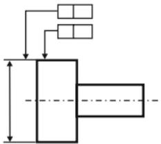
Indicating arrow as an extension of the dimension line: if the tolerance applies for the axis or median plane or a point of the element.
