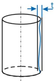
The tolerance zone is limited by two parallel lines at a distance  $t$  apart. Every envelope line of the tolerated cylinder must be between these two parallel lines.
