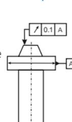
Every circle line of the tolerated area must be between two parallel circle planes at a distance apart of 0.1 with their common center point on the datum axis A.
