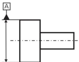
Restriction of the datum to an area of the element as a dot-dash line with dimensioning.
