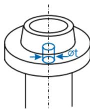
The tolerance zone is limited by a cylinder of diameter  $t$ , the axis of which matches the datum axis. The actual axis of the tolerated element must be within the tolerance zone.
