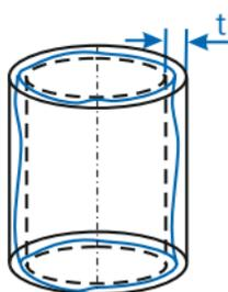
The tolerance zone for the cylinder envelope area limits the deviation of the roundness, the straightness of the envelope line and the parallelism of the envelope line to the cylinder axis. It is formed by two coaxial cylinders with the radial distance  $t$ .
