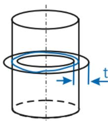
The tolerance zone is limited by two concentric circles at a distance  $t$  apart. The circumference line of the tolerated cylinder must be within a circle ring of the zone width  $t$ , in every radial section plane.
