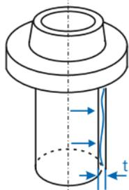
The tolerance zone within which the envelope lines of the tolerated cylinder must lie is limited by two parallel lines at a distance  $t$  apart which run parallel to the datum plane.
