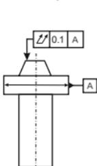
The tolerated area must be between two parallel circle planes at a distance apart of 0.1 with their common center point on the datum axis A.
