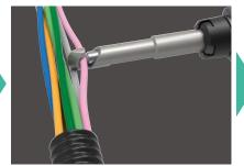
Hook the open end to the CAN bus
