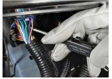
Quickly pinch with one hand from over the sheath
