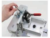
Pull the lock lever toward you to allow the probes to be lowered. This design keeps the probes from being lowered inadvertently.
