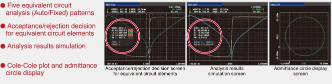
Equivalent Circuit Model and Measurement Items
