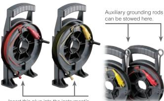
Insert this plug into the instrument's S(P)/H(C) terminal and pull out the cord.
