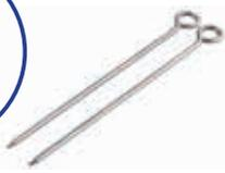
Since variations in the thickness of auxiliary grounding rods cause almost no change in their grounding resistance, the FT6031-50 uses thinner rods that are easier to drive into the ground.
