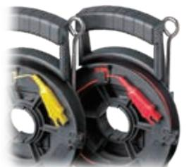
Insert this plug into the instrument's S(P)/H(C) terminal and pull out the cord.
