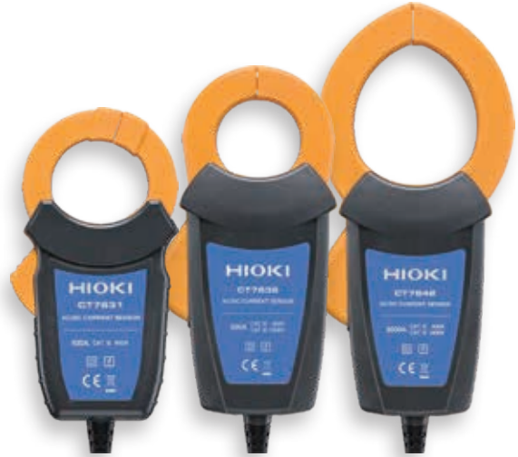
CT7631 AC/DC100A φ33mm (1.3 in) CT7636 AC/DC 600A φ33mm (1.3 in) CT7642 AC/DC 2000A φ55mm (2.17 in)
