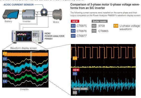
CT687x current sensors can accurately measure currents that were hidden by noise when observed with earlier models because they are not affected by noise that accompanies switching at a high carrier frequency (FSW: 100 kHz).
