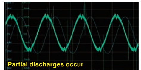
Current and voltage waveforms when 1.5 kV AC is applied to a non-defective stator
