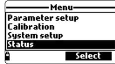
Select "Meter Status" to display information related to the battery, logging, internal temperature, password, Meter ID, serial number and firmware version.
