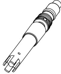
**HI7698194-1** Combination pH/ORP sensor features a glass sensitive bulb for pH readings, a platinum sensor for redox measurements and a silver/silver chloride double junction reference with gelled electrolyte.
