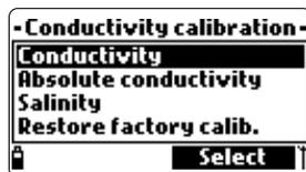
*Note: To improve accuracy, choose a calibration standard near the sample conductivity.*
