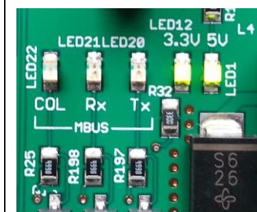
The COL LED indicates overloading or data collision within the M-BUS network.
