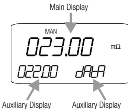
The main display appears immediately after the milliohm-meter is switched on, but the auxiliary displays have to be activated by pressing the DATA|CLEAR key.
