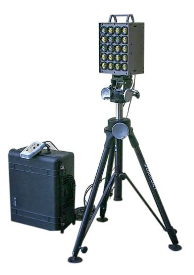
The UVTS is a short to long-range electro-optical missile threat simulator for testing missile approach warning systems and training crew in the operation of these systems. It simulates the UV radiation profile of an approaching missile
