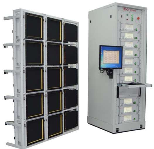
Figure 10: "NUC Tower" System with 15 controlled temperature blackbodies
