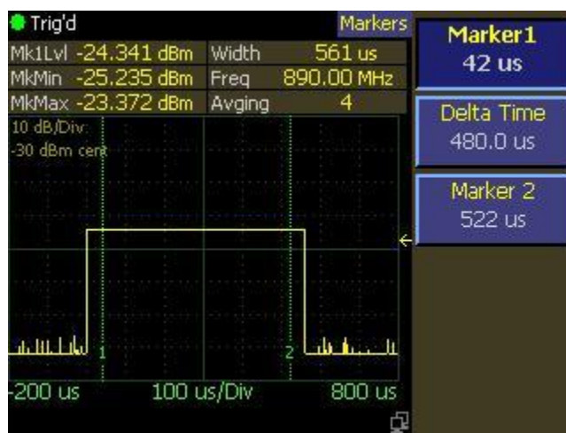
Figure 3-7 GSM Signal with Marker Measurements
