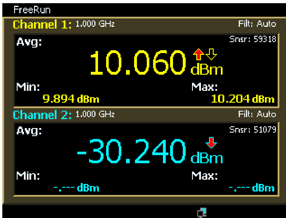
Fig. 4-26A Text Display with Alarm Over-range and Under-range Arrows. (The outline arrow indicates a previous alarm condition that has cleared.)
