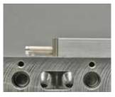
Detector retracts during standby and after measuring
